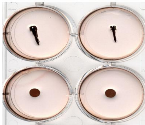
Figure 9. Specimens in the agar overlay assay. Cytotoxic activity would induce decoloration of the cells under and next to the specimen. A decolorized zone would be apparent macroscopically- Finke C et al (2018) 22
