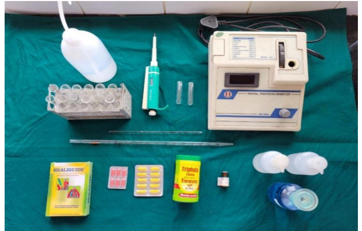
Figure 1. Depict the armamentarium of the current study that shows the Healiguide membrane, doxycycline (Yellow tablets), Tetracycline (pink tablets), Triphala Churna box, collagenase enzyme, photo-colorimeter, micropipette (green colour), cuvettes etc.
