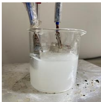
Figure 2. Coating of Mg alloy with Chitosan-Bioactive Glass at 0.10V, 0.05A.
