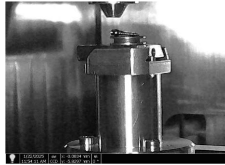
Figure 1. Showing mini-screw implants mounted on aluminium supporting discs using double carbon sided tape under the microscope.
