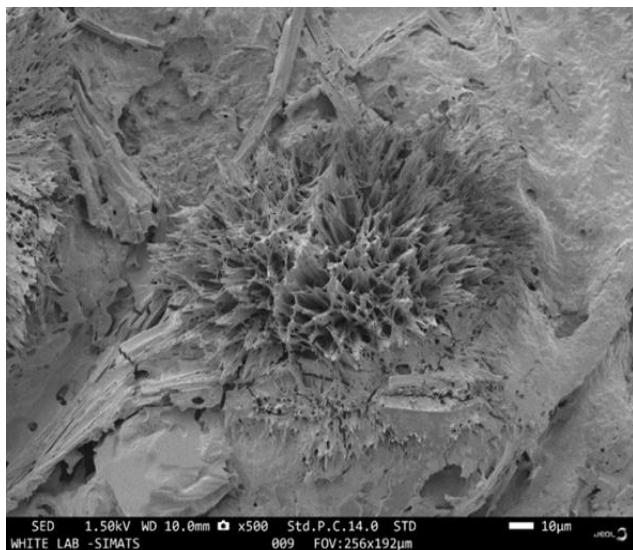
Figure 3. SEM analysis of erbium-doped HA/Bioglass-PVA scaffold under 500X magnification
