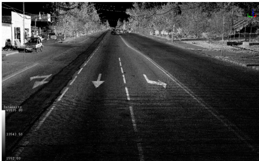
Fig. 2. Point cloud generated from scanning, incorporating intensity values.
